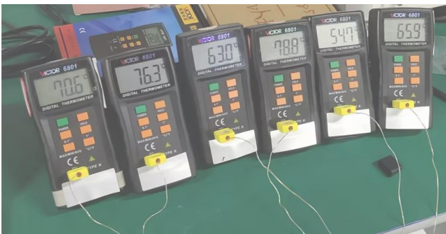
Fig.7 SIC hybrid scheme thermocouple test
